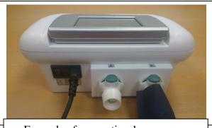
Example of connection 1 accessory: Sleeve In this case the unused track must be closed with a plug (supplied)
